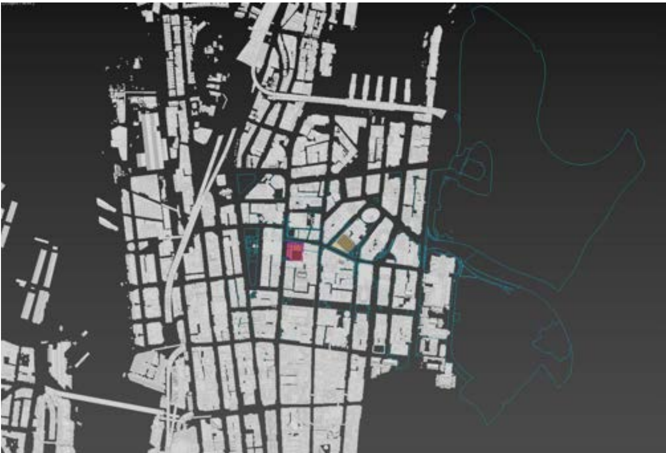
Image showing 3D building model (red and yellow) aligned to survey drawing from RPS (blue), as well as Sydney AAM model (White) by aligning site boundary of the Metro East and West locations
